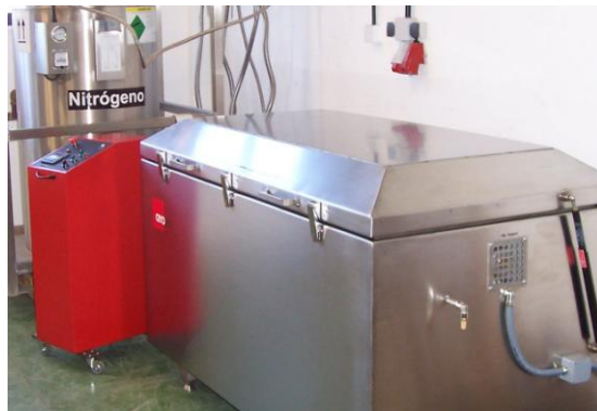
Figure 1: Multistage cryogenic processor designed and manufactured by Cryobest International, S.L.
