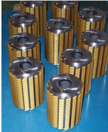
Figure 3: Insert blade hobs after a multistage cryogenic treatment.
