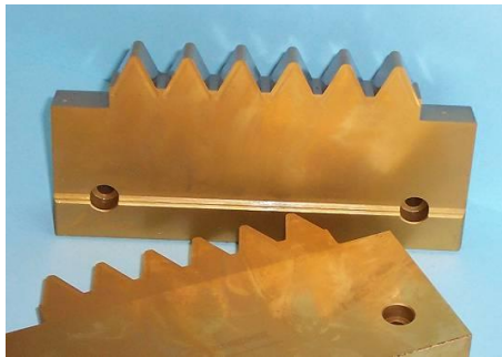
Figure 2: Maag type cutters (TRW, Spain)
